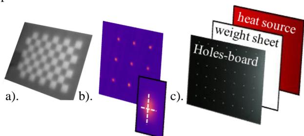
Figure 1: a). Chessboard image by LWIR camera using constant illumination. b). Image of holes-board by LWIR and the result of ellipse center location analysis of one hole. c). Holes-board with white sheet and heat source object constalation
